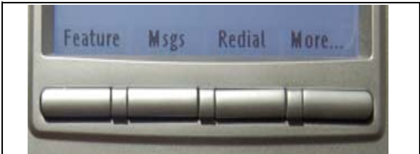
Figure 4: Context-sensitive soft keys when the IP Deskphone is in the idle state
